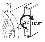
Allow the Engine to run for several seconds. Then, if the Choke lever is in the CHOKE position, move the Choke Lever very slowly to its RUN position.
