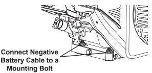
6. Coat the terminals and cable ends with a corrosion-preventive coating.
