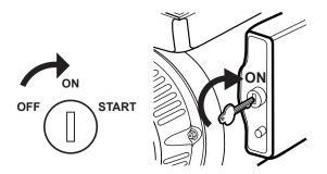
b. Grip the Starter Handle of the Engine loosely and pull it slowly several times to allow the gasoline to flow into the Engine's carburetor. Then pull the Starter Handle gently until resistance is felt. Allow Cable to retract fully and then pull it quickly. Repeat until the engine starts. Note: Do not let the Starter Handle snap back against the engine. Hold it as it recoils so it doesn't hit the engine.
